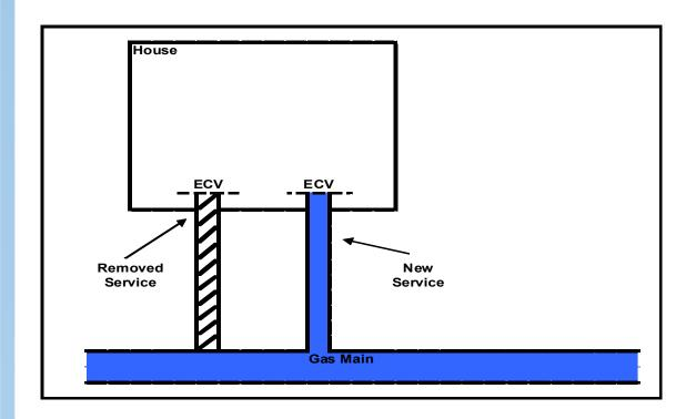
Old service disconnected and new service fitted at a different location in the gas main
