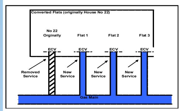
House converted to flats old service removed and additional services fitted at different points in the same gas main
