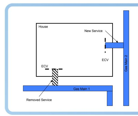
Old service disconnected and new service fitted at different main.
