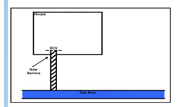
New service laid at any point on the main (New Development – Could be a plot addess)
