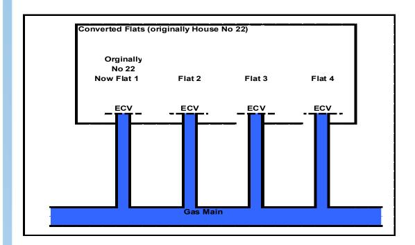
House converted to flats and existing service changed to flat 1 and additional services fitted at different points in the same gas main.
