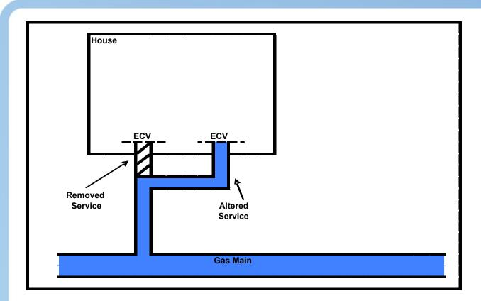
Service laid at same point on the main (Alteration of service, Service replacement & Capacity increase)
