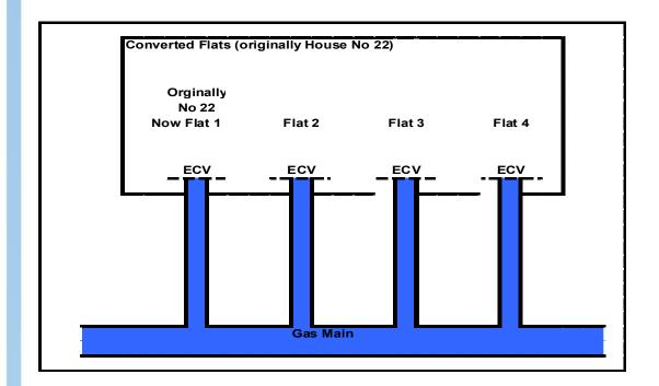
House converted to flats and existing service changed to flat 1 and additional services fitted at different points in the same gas main.
