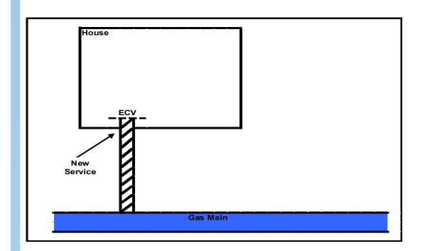
New service laid at any point on the main (New Development – Could be a plot addess)
