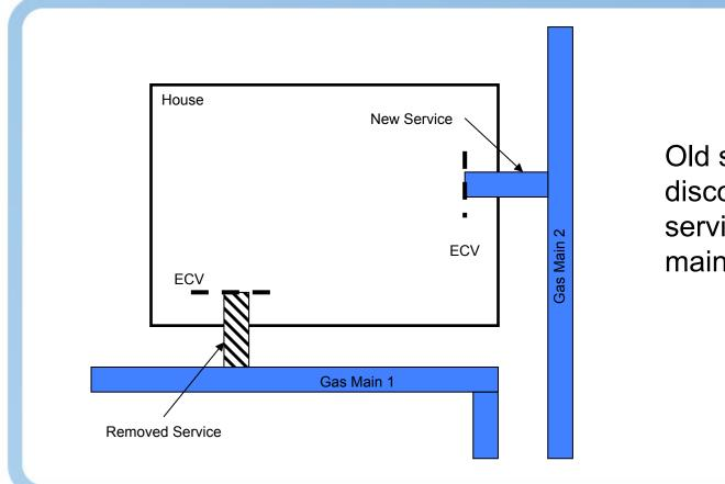
Old service disconnected and new service fitted at different main.
