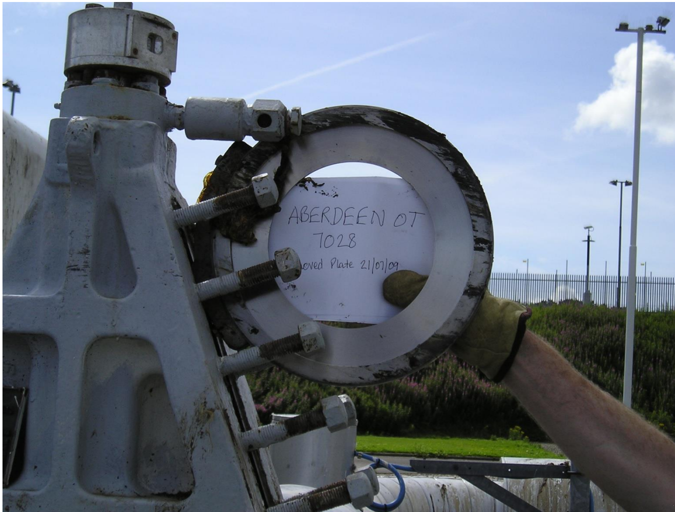
Figure D.1 – Orifice Plate (“As Found”) 21 st July 2009
