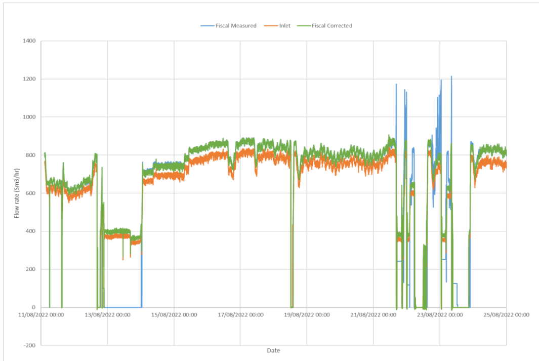
Figure 2 Volume flowrates for Fiscal USM, Inlet USM and corrected Fiscal USM
