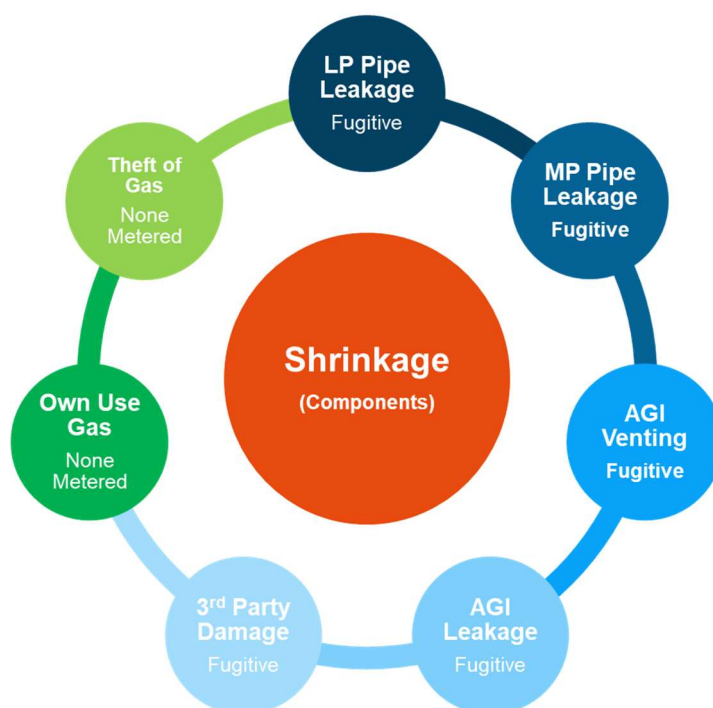
Figure 6 Seven Components of Shrinkage
