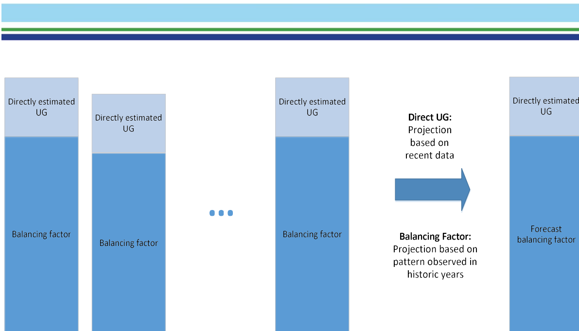
Figure 5: Projecting Unidentified Gas
